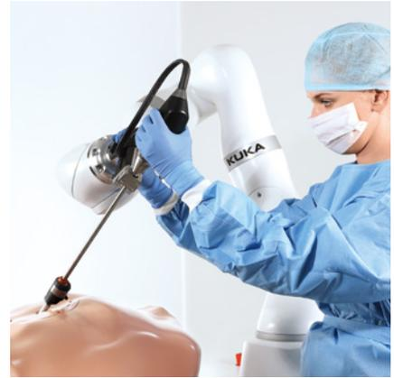
**Minimally invasive surgery:** The highly developed controller enables precise operation with a trocar kinematic system. The user can freely select whether to use the application automatically, interactively or via a telemanipulator.
