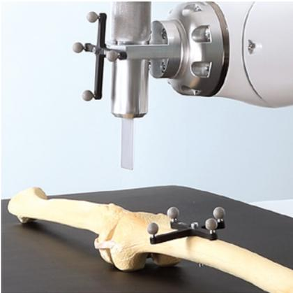
**Orthopedic surgery:** Thanks to its stable design and construction, as well as its high stiffness, the LBR Med is suitable for bone surgery. Open-source libraries facilitate the fast development of prototypes and the integration of navigation cameras.
