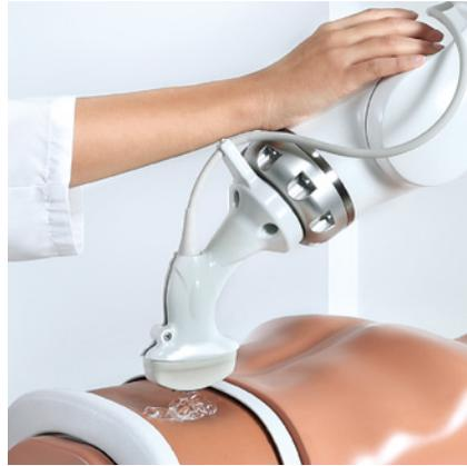
**Ultrasound diagnostics:** Sensitive technology and safe human-robot collaboration are the domain of the LBR Med. Thanks to the integrated sensors, it can react to its surroundings both interactively with the physician and via telemanipulation.
