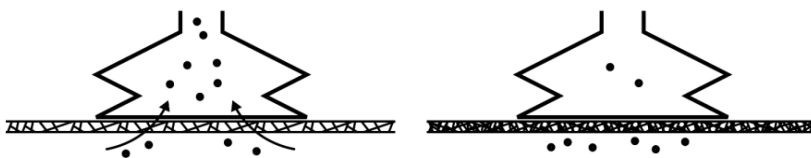
Figure 3.6: Visualization of difference in leakage through workpieces.
